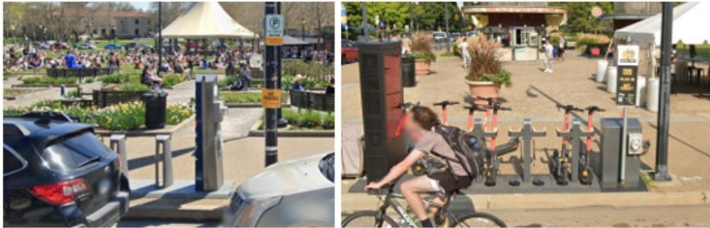
Schenley Plaza mobility hub in Pittsburgh, Pennsylvania, leveraging no-trench connections to city-owned lampposts for electric bike-share and scooter stations, according to email correspondence with the Pittsburgh Department of Mobility and Infrastructure. Source: Google Maps Street View
