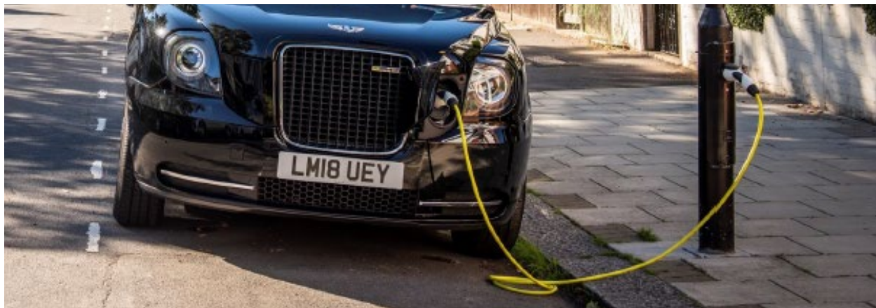
Ubitricity bollard charging station in the UK. Source: Ubitricity
