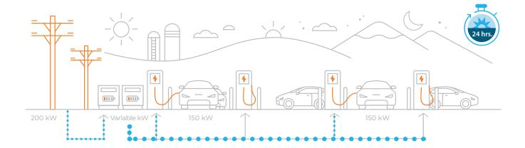
**DESIGN DAY:** The Design Day is the heaviest day of charging energy demand that the station is intended to serve without interruption to service due to a depleted battery—for example, the 99th percentile day in 2030. The selection of an appropriate Design Day is crucial for right-sizing an energy storage system. To reliably meet charging demand on the Design Day and recharge itself, the battery-buffered DCFC must achieve two things:
